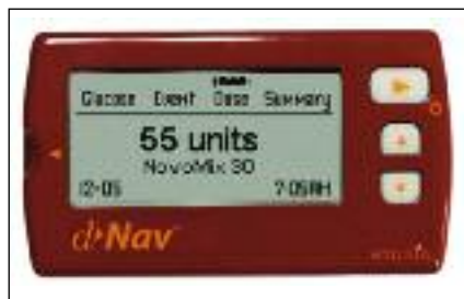
Figure 1. The handheld d-Nav insulin guidance device. d-Nav is used to check capillary blood glucose and, based on the identification of patterns in time-tagged glucose readings, provides insulin dosage guidance on a weekly basis or more frequently in the presence of hypoglycaemia or near hypoglycaemia
